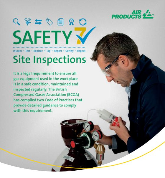
Code of Practice 47 (CP47) details the tests for single cylinder systems, and Code of Practice 7 (CP7) details the testing specifically for oxy-fuel equipment, including regulators and flashback arrestors.
